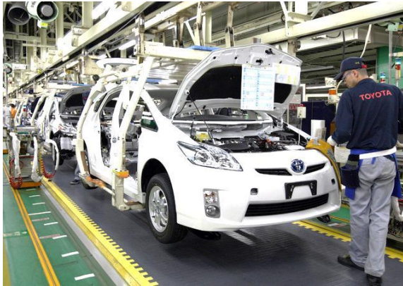
Figure 1. The Toyota production system, where all employees are empowered to stop the production line for any reason
